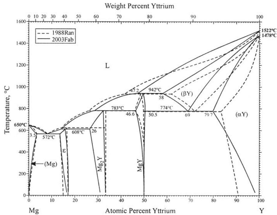
**Fig. 1** Mg-Y phase diagram
